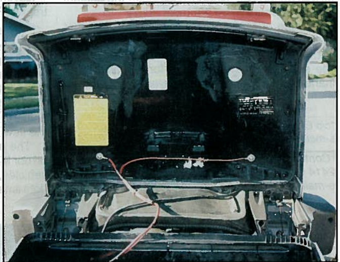
Photo C—Ray has mounted all of his radios in the rear of his bike, putting only remote heads up front.
