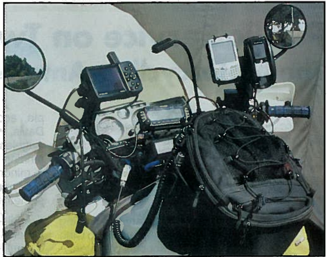
Photo B—Radios and other devices, such as GPS receivers and personal digital assistants, are mounted to be safe yet in easy view.
